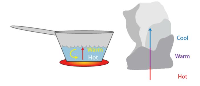
Transfer of thermal energy through circular motion caused by heating and cooling in fluids (liquids and gases)
